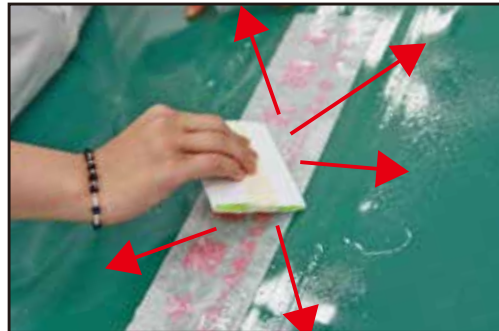
⑤ Start from the middle and work towards the edges, applying pressure with the squeegee to remove the water.
