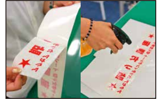
③ Peel off the mounting sheet and use the spray bottle to wet the adhesive side.
