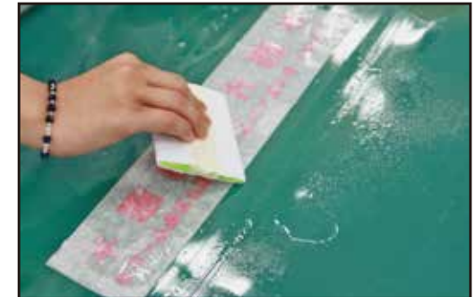
⑥ Rub the surface with the squeegee until all the water is completely removed from under the vinyl letters.
